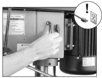
Figure 27. Using the belt tension lever.
